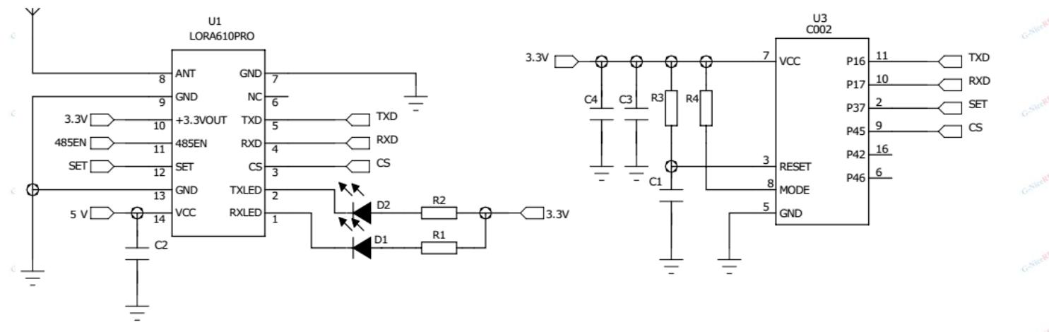
Note: The ground wire of the module must be connected to the digital ground of the device.
